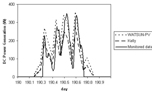
Figure 4. DC Power generation of Array A on July 9
