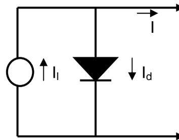
Figure 1. A one-diode equivalent circuit.
