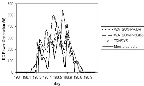
Figure 12. DC Power generation of Array A on July 9
